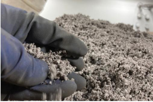
FIG. 3: Given the surface area, the total coal slag abrasive media (top) required for this job was estimated to be 21 to 22 semi-trucks filled with abrasive media. After test blasting determined that 100 lbs. of coal slag removed just under 1 square foot of coal-tar enamel, it was apparent that sponge media (bottom), along with robotic abrasive blasting, was the only viable option.
