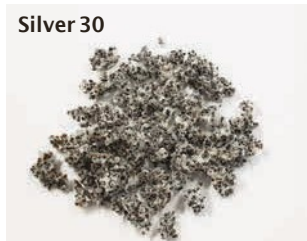
At BERNMOBIL we currently use Silver 30 Sponge Media and Silver 60 Sponge Media. Both are abrasive.
