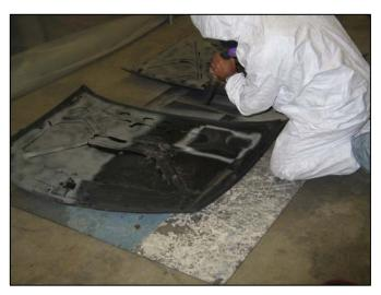
Figure 1 - Abrasive blasting with composite abrasives during 2nd test series. Note the absense of visible airborne emissions during blasting. *Photo coutesy of Midwest Research Institute.*
