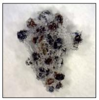
Figure 20 – Particle of composite abrasive, bonded with 30-Grit Aluminium Oxide. *Photo coutesy of Sponge-Jet, Inc.*
