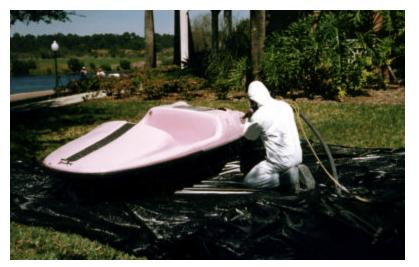
An amusement park needed to strip and repaint selected runabouts. Subject to harsh sun and the marine environment, the runabouts were removed from water, stripped, painted and promptly returned to service. Maintenance personnel chose to test the Sponge Blasting System to strip 20 to 40-mil of marine epoxy from the boats, creating a less-than-one mil profile and causing no further damage to the sensitive gel-coat base.
