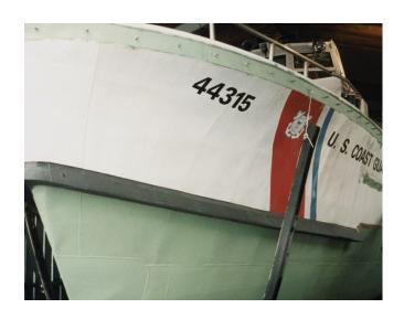
The need for a dry, low dust, reusable, abrasive blasting technology was the reason a U.S. Coast Guard Industrial Support Detachment switched to using the Sponge-Jet Sponge Blasting System for surface preparation. In place of using coventional abrasives, they now Sponge Blast their 41,44,46,47 and 55 foot Patrol Boat interiors and exteriors. This Industrial Support Detachment uses Silver Sponge Media™ abrasives to remove an average of ten mils of epoxy topcoat and primer.
