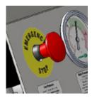
Location and usage of Emergency Stop Button should be understood before operation. Pushing in the Emergency Stop Button stops operation;
