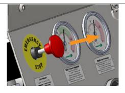
Confirm **Media Feed Pressure** Gauge reads consistently with **Typical Media Feed Pressure** label on Unit or in chart below.
