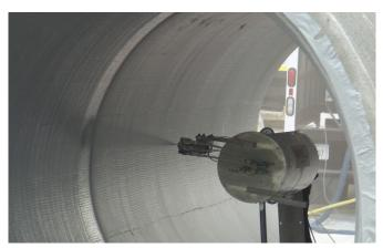
ABOVE - Meanwhile, another robotic cart designer Mike Kronz tested his machine inside a plywood pipeline mockup at his facility, also in Wisconsin. His goal was to pair his robotic cart with a Graco Probler P2 Elite internal mix gun to see how efficiently he could install polyurea onto epoxy pipe, on a test basis.
