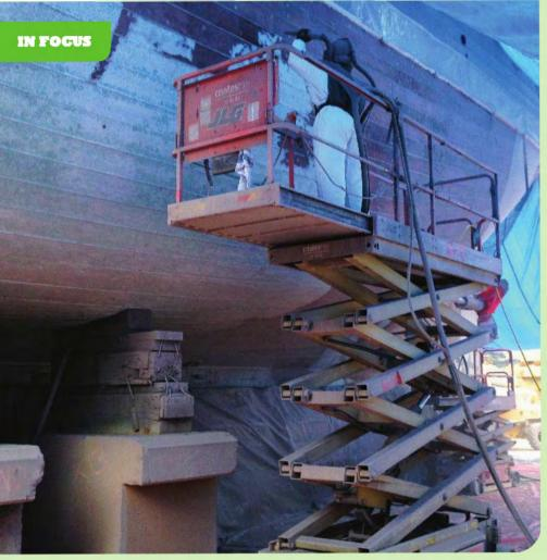
typically associated with conventional blasting. This not only saved the time and money, but allowed other trades to work near the blast operation without unnecessary exposure to airborne dust, which in most instances contains a variety of unhealthy residues. Encapsulated media also scored high marks in removing chloride and other contaminants.
