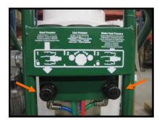
Confirm Manual Rotation Knob is rotating, Air Motor Lubricator rate is 1-2 drops per minute.
