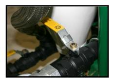
3. Remove **Clean Out Trap**; rotate **Manual Rotation Handle** clockwise and counter-clockwise until obstruction falls out. **Auger** should move smoothly. Replace **Clean Out Trap**.
