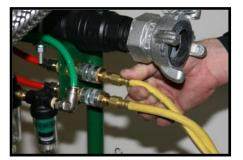
Check **Main Air Ball Valve** and **Accessory Air Supply Valve** are closed. Charge supply line from air source.
