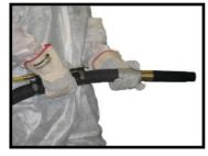
Set **Media Feed Pressure** to 0.7bar(10psi) and adjust as required.
