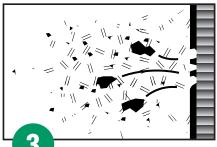
Conventional abrasives release all fractured abrasives, contaminants, and coating layers as airborne dust
