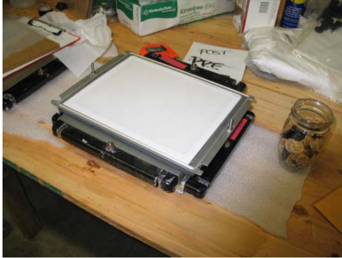
Photo 7. Exposed Filter for Test Substrates Shown in Photos 6a and 6b
