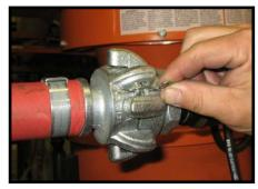
Adjusting Frame Height: Remove Frame Height Locking Pin (both sides)
