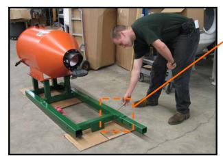
Insert the **Frame Height Locking** pin,
