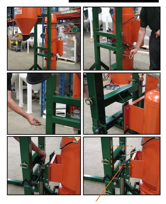
Tighten jack before raising frame to desired height
