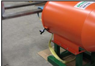
Lifting strap should be rated minimum 453kg (1,000lbs)
