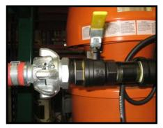
Connect a minimum 32mm (1.25in) supply hose to **Supply Line Connection**. **Note:** High humidity environments require additional moisture separators.
