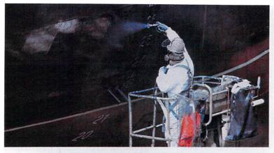
After being spot-blasted and sweep-blasted with a water ring attached just behind the blast nozzle, the trawler's freeboard gets a high-gloss, UV-resistant top coating of Proline 4800 in Alaska Ocean Seafood Blue.
